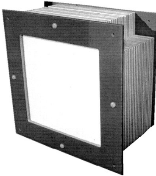
Figure 9. Realization of a negative epsilon structure: photograph of the structure shown in figure 8. The aperture is 200 mm × 200 mm.
